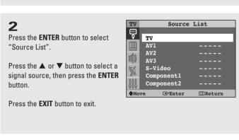
■ When you connect equipment to the TV, you can choose between the following sets of jacks: "AV3", "S-Video" on the TVs side panel or "AV1", "AV2", "Component1" or "Component2" on the TVs rear panel.
